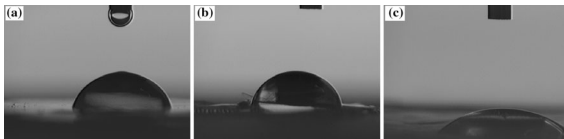
Fig. 7 Microphotographs of water dripping experiment on different film surface: a pristine DFMA73 film, b corona-treated DFMA73/TiO 2 film, and c acrylic acid surface-grafted DFMA73/TiO 2 film
